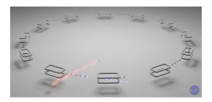
GF concept: laser photons (pink waves) are scattered by PSI circulating in an accelerator ring. The scattered photons propagate in the direction of the ions motion (purple arrows) - resulting in an intense beam of highly energetic gamma rays. Credit: Universitaet Mainz
