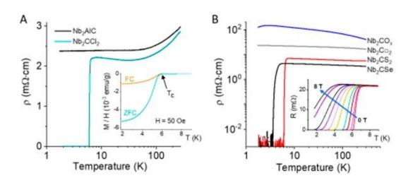
Electronic transport and superconductivity in Nb2CTn MXenes. (A) Temperature-dependent resistivity for the cold-pressed pellets of Nb2AlC MAX phase and Nb2CCl2 MXene. (Inset) Magnetic susceptibility of Nb2CCl2 MXene as a function of temperature. FC and ZFC correspond to the field cooled and zero-field cooled measurements, respectively. (B) Temperature-dependent
