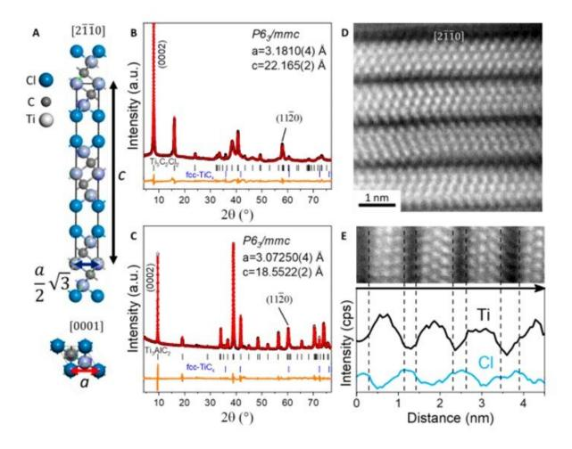
Structure of Ti3C2Cl2 MXene. (A) The structure of Ti3C2Cl2 MXene can be approximated using P63/mmc space group with the two lattice parameters: inplane, a, and out of plane, c. Experimental XRD patterns (Cu K $\alpha$ , reflection, black curve), Le Bail fits (red curve) and the corresponding residues (orange curves) of (B) Ti3C2Cl2 MXene derived from (C) Ti3AlC2 MAX phase. The successful MXene synthesis can be visualized from the shift of (0002) and
