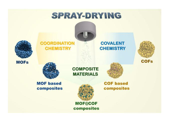
Diagram of the different materials that can be obtained with spray-drying. Credit: ICN2
