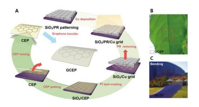
Figure 1. Electrode platform consisting of CEP film and a GCEP. (a) The GCEP fabrication process and (b, c) digital images of GCEP. Credit: Ulsan National Institute of Science and Technology
