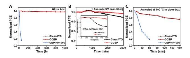
Figure 2. Stability of PSCs based on GCEP. Normalized PCE degradation under (a) storage, (b) continuous illumination at 1 sun condition without UV-pass filter (and at 12 sun condition with UV-pass filter (inset)), and (c) heating at 100 °C, always in a N<sub>2</sub>-filled glovebox. Credit: Ulsan National Institute of Science and Technology
