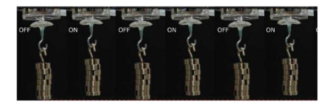
Series of protein-based artificial muscles, with performance exceeding that of biological muscle. Other soft robotic parts could include soft grippers and soft actuators. Credit: Demirel Lab, Penn State
