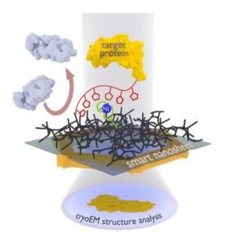
The protein complex to be examined (yellow) is attached to the smart nanosheet via a nickel complex with the aid of a marker (red chain with pentagons). Unwanted proteins (gray) are repelled by the hydrogel (black grid). After freezing the entire structure, including a thin film of water, this can be irradiated with electrons to obtain images of the bound proteins, from which a computer can then calculate the 3D structure of the protein. Credit: Andrey Turchanin/Zian Tang
