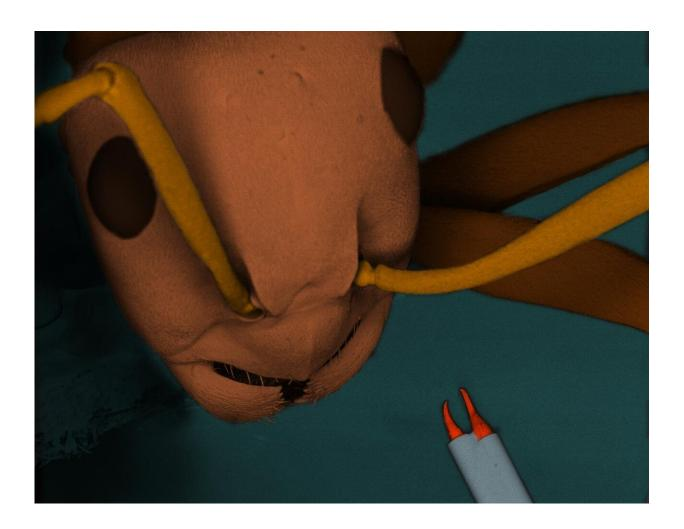
The optical pliers next to the mandibles of a Formica polyctena ant for comparison (composite scanning electron microscope (SEM) image with added colors). The two jaws (red) close when light is sent through the optical fibers (light blue) that have the diameter of 125 microns, comparable to the diameter of a human hair. (Source: UW Physics) Credit: UW Physics
