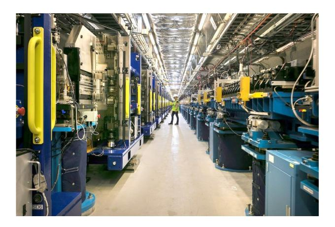
A worker inspects the soft X-ray undulator at SLAC National Accelerator Laboratory. The hard X-ray undulator is visible at right. (Credit: SLAC National Accelerator Laboratory)
