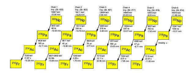
Fig. 1. Correlated  $\alpha$ -decay chains of  $^{222}$ Np observed in the present work. Credit: IMP
