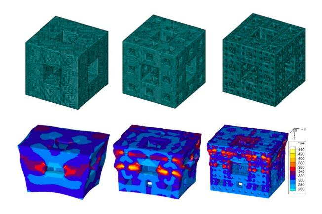
Simulations show how fractal structures of increasing complexity dissipate energy from shockwaves. Credit: Los Alamos National Laboratory
