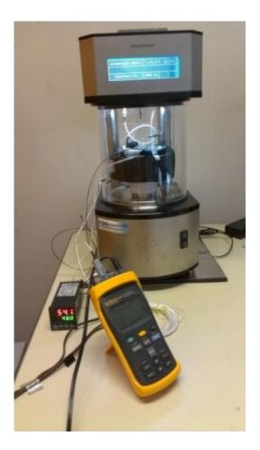
The team measured surface tension in seawater ranging from room temperature to 90 degrees Celsius and salinity levels ranging from pure water to four times the salinity of ocean water. Credit: Kishor Nayar
