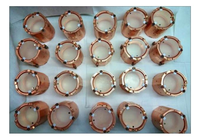
CUPID-Mo's 20 cylindrical crystals are pictured in their copper casing. Credit: CUPID-Mo collaboration
