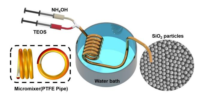
Experimental set-up of the microfluidic mixer for the synthesis of silica. Credit: Yang Hui
