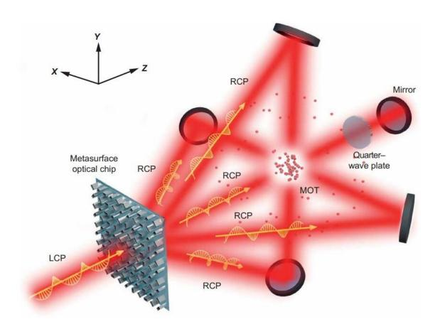
Schematic of the cold atom device with the dielectric metasurface optical chip. Credit: *Science Advances* (2020).
