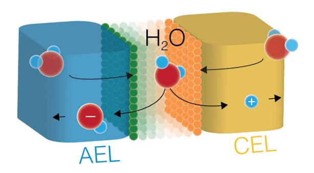
Research in a University of Oregon chemistry lab has advanced the effectiveness of the catalytic water dissociation reaction in bipolar membranes. A three-member team used a membrane-electrode assembly where the polymer bipolar membrane is compressed between two rigid porous electrodes, allowing them to make a large number of bipolar membranes with different water dissociation catalyst layers. Credit: Sebastian Z. Oener
