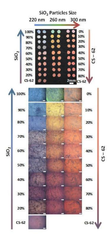
In their study, the researchers proposed structural color printing using simply binary mixtures of particles to produce a broad gamut of saturated structural colors. Credit: University of Akron
