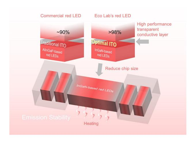
The team developed an InGaN red LED structure where the output power is more stable than that of InGaP red LEDs. Credit: Zhe Zhuang
