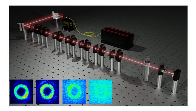
Experimental setup for the realization of arbitrary VVB and OAM modes for the analysis of spatial and polarization properties after the interaction with a scattering media constituted by a water solution of micrometrical latex beads. Inset: spatial modes of light carrying orbital angular momentum through increasing concentrations of scattering media. Credit: Gianani et al., doi 10.1117/1.AP.2.3.036003.
