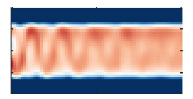
Sound propagating in a two-dimensional Fermi gas. The image shows the density of the gas in time, shortly after a sound wave has been excited. Dark red values correspond to a high density, lighter values to a low density. One can see a wave traveling up and down between the boundaries of the gas multiple times as time progresses to the right. Not shown: The damping of the sound wave is lowest where the particles of the gas interact most strongly. Credit: Bohlen et al.
