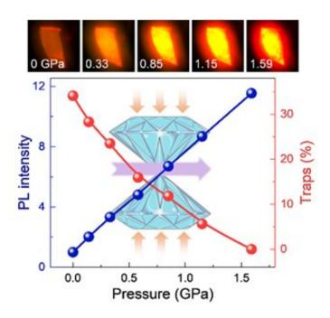
Fluorescence micrographs during compression and the PL intensity and contribution of the trapped states' emission as a function of pressure. Credit: Center for High Pressure Science & Technology Advanced Research
