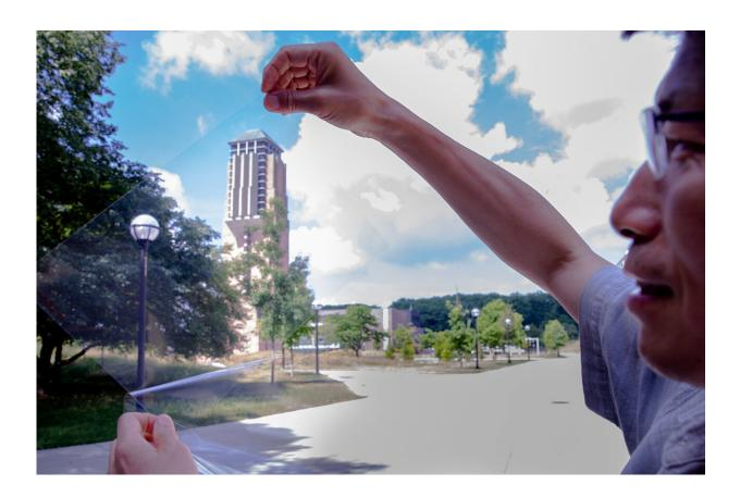
Jay Guo holds a sheet of flexible transparent conductor on the University of Michigan's College of Engineering North Campus. The material sandwiches a thin layer of silver between two "dielectric" materials, aluminum oxide and zinc oxide, producing a conductive anti-reflection coating on the sheet of plastic. Photo by Robert Coelius/Michigan Engineering
