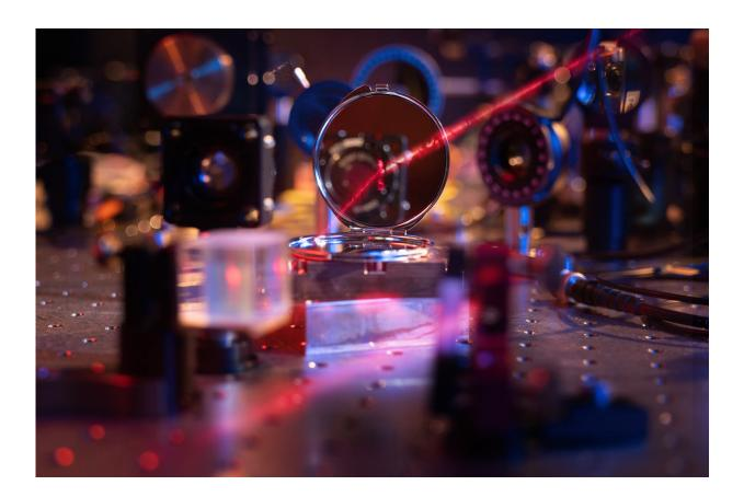
Researchers have demonstrated a novel light-matter interface, realizing the lightest possible mirror formed by a monolayer of 200 atoms. Credit: Max Planck Institute of Quantum Optics
