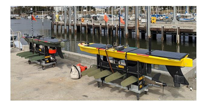
During the Summer 2020 CANON experiment, these two Wave Gliders have been zig-zagging over Monterey Canyon, using echosounders to locate fish and other animals in the water below. The echosounders are the cylindrical devices near the back of each Wave Glider. The olive-green foils under the Wave Gliders help propel these autonomous robots across the sea surface. Credit: Chris Wahl/MBARI
