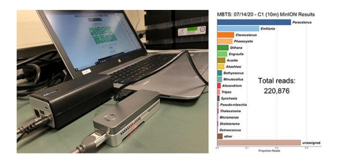
During the Summer 2020 CANON experiment, researchers are testing small "benchtop" DNA sequencers that plug directly into a laptop computer. After analyzing one water sample, the sequencer produced a graph showing how much DNA was detected from different types of animals, including anchovies, copepods, and microscopic algae. Credit: Charles Nye/MBARI
