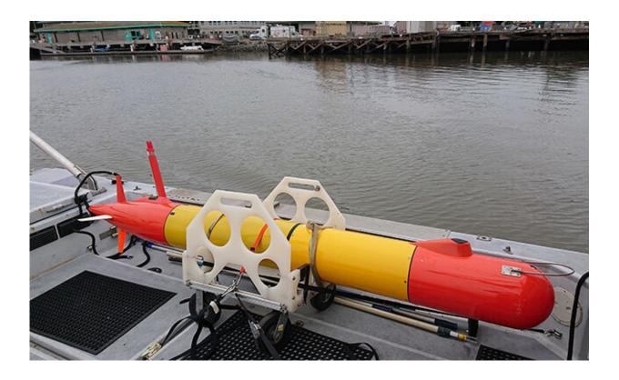
Inside of this underwater robot (a long-range autonomous underwater vehicle or LRAUV) is a robotic laboratory called an Environmental Sample Processor, which collects samples of seawater then extracts environmental DNA for later analysis onshore. Credit: Erik Trauschke/MBARI
