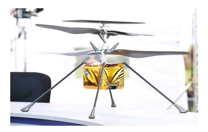
Once on the surface, NASA will deploy the Ingenuity Mars Helicopter—a little 1.8 kilogram (four pound) aircraft that will attempt to fly in an atmosphere that is only one percent the density of Earth's
