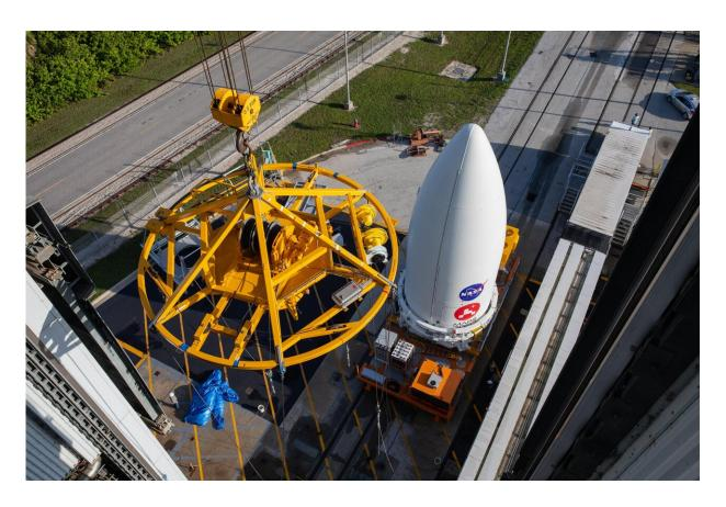
A crane stands at the ready to hoist the payload fairing, or nose cone, containing NASA's Mars 2020 Perseverance rover onto the top of an Atlas V launch vehicle. The image was taken at the Vertical Integration Facility at Space Launch Complex 41 at Cape Canaveral Air Force Station in Florida on July 7, 2020. Credit: NASA/KSC
