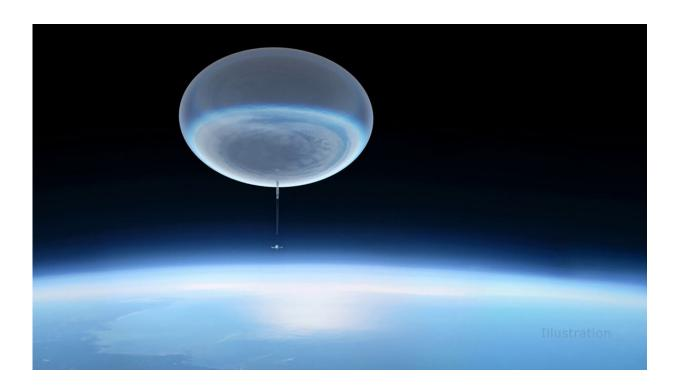
This illustration shows a high-altitude balloon ascending into the upper atmosphere. When fully inflated, these balloons are 400 feet (150 meters) wide, or about the size of a football stadium, and reach an altitude of 130,000 feet (24.6 miles or 40 kilometers). Credit: NASA's Goddard Space Flight Center Conceptual Image Lab/Michael Lentz
