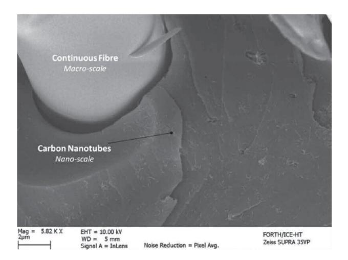
Scanning electron microscope image of multi-scale reinforced composite showing the different scales involved, with macroscopic carbon fibre and nanoscale carbon nanotubes. Credit: Adamant Composites
