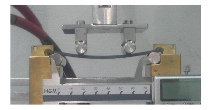
Testing the strength of nano-material-augmented composite diving fins by flexing them. Credit: Alchemy
