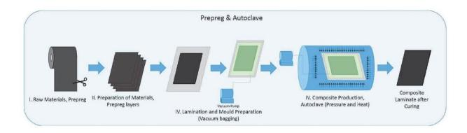
Prepreg/autoclave composite manufacturing: process steps. Credit: Adamant Composites
