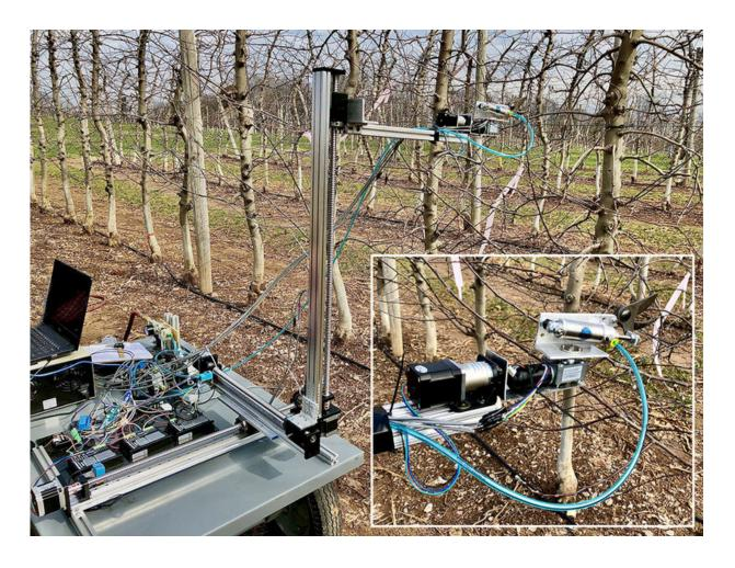
The end-effector prototype in action at Penn State's Fruit Research and Extension Center in Adams County, Pennsylvania. There were major challenges to creating a mechanical system that would succeed in a complex agricultural environment, according to researchers. The robotic cutting unit had to be able to operate in tight spaces and reach targeted branches for pruning while avoiding the tangle of other branches. Credit: Long He research group, Penn State
