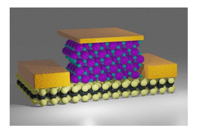
Calcium fluoride is a crystalline insulator with a well defined surface. Therefore, it is ideally suited for manufacturing extremely small transistors. Credit: Vienna University of Technology
