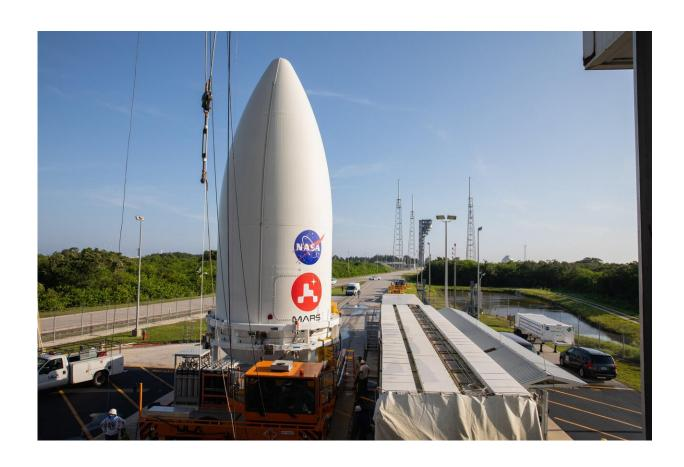
The nose cone containing the Mars 2020 Perseverance rover sits atop a motorized payload transporter at Cape Canaveral Air Force Station in Florida on July 7, 2020. Credit: NASA/KSC
