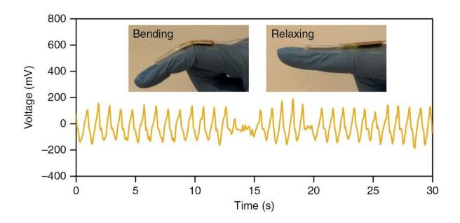
Output voltage in a practical, wearable device: voltage output during tensile bending and relaxing (two-electrode device). Credit: FLEET
