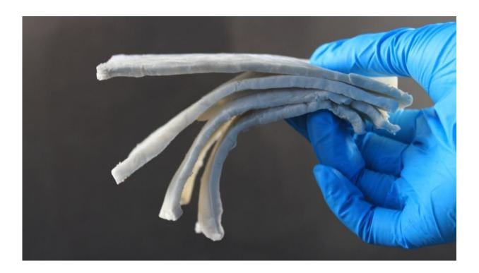
A sample of the electromagnetic shielding material made by Empa – a composite of cellulose nanofibres and silver nanowires. Credit: Empa
