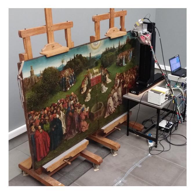
The MA-XRF instrument during experiments on the central panel (Adoration of the Lamb). Credit: University of Antwerp
