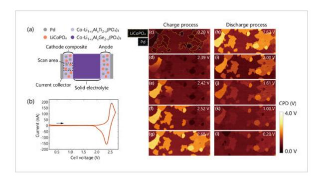
Changes in electrical potential distribution across a composite cathode during charge (a–f) and discharge (g–l) processes. Credit: National Institute for Materials Science
