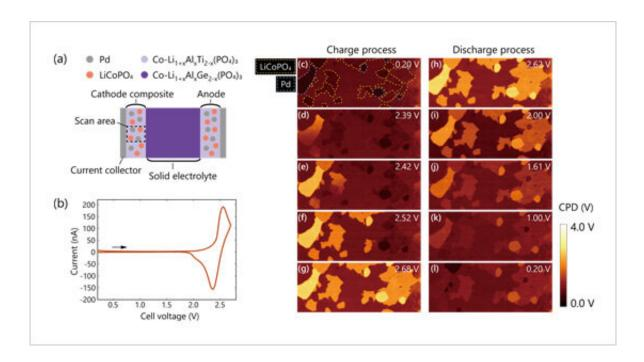
Changes in electrical potential distribution across a composite cathode during charge (a–f) and discharge (g–l) processes. Credit: National Institute for Materials Science
