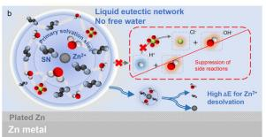
Schematic diagrams of Zn<sup>2+</sup> solvation structure and interfacial reactions in (a) traditional aqueous electrolyte and (b) hydrated eutectic electrolyte. Credit: Zhao Jingwen and Yang Wuhai
