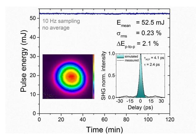
Long term stability of the Ho:YLF chirped pulse amplifier at a 1 kHz repetition rate. The average pulse energy Emean=52.5 mJ was measured over a period of 120 minutes. The standard deviation has a value of  $\sigma$ rms=0.23%, the pulse-to-pulse energy fluctuations are  $\Delta$ Ep-to-p=2.1%. Left inset: Beam profile (far-field intensity distribution). Right inset: Autocorrelation trace of the re-compressed 52.5 mJ pulses, measured and simulated. Credit: MBI
