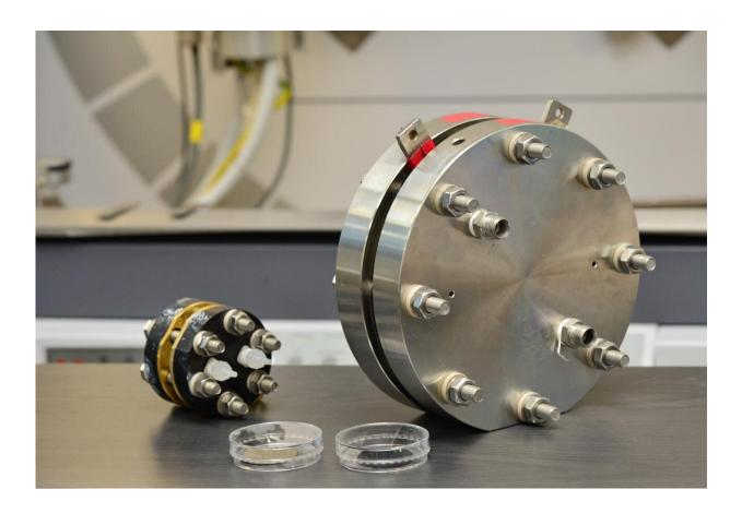
(Right) Coral shape silver nano-catalyst electrode with high-performance, largearea developed by KIST researchers (electrode size 50 cm) (Left) Catalyst electrode for synthetic photosynthesis in existing gas state (electrode size 2cm) Credit: Korea Institue of Science and Technology(KIST)
