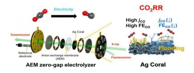
Coral-shaped schematic diagram of carbon dioxide conversion systems using electrodes Credit: Korea Institue of Science and Technology(KIST)
