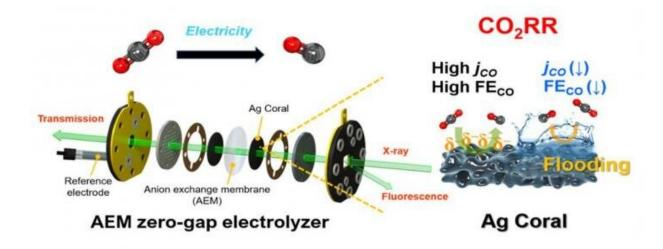
Coral-shaped schematic diagram of carbon dioxide conversion systems using electrodes Credit: Korea Institue of Science and Technology(KIST)
