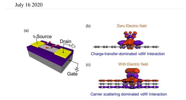
(a) Adsorbed CO2 molecules on graphene sensor (b) van der Waals (vdW) interaction between adsorbed molecules and graphene at zero electric field (c) vdW interaction between adsorbed molecules and graphene with electric field. Credit: JAIST
