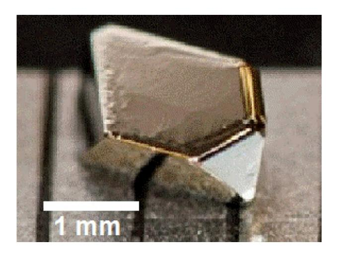
This image shows an example of a crystal of iron sulfide grown in the University of Minnesota lab to extremely high purity using a method called chemical vapor transport. Note the "goldish" sheen, which is characteristic of pyrite, or fool's gold. Credit: University of Minnesota
