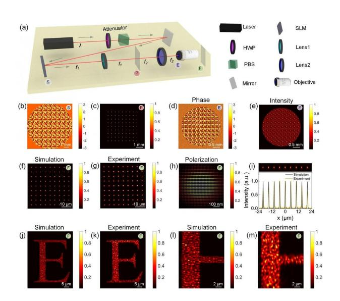
(a) Sketch of the optical system. (b) CGH displayed on the SLM for the generation of a 9×9 foci array. (c) The foci array on the focal plane of Lens 1 (P plane). (d) Phase distribution and (e) intensity distribution on the entrance pupil
