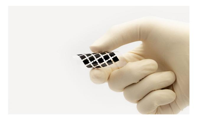
Single-crystal perovskite films could enable more efficient flexible solar cells such as the one pictured here. Credit: Yusheng Lei
