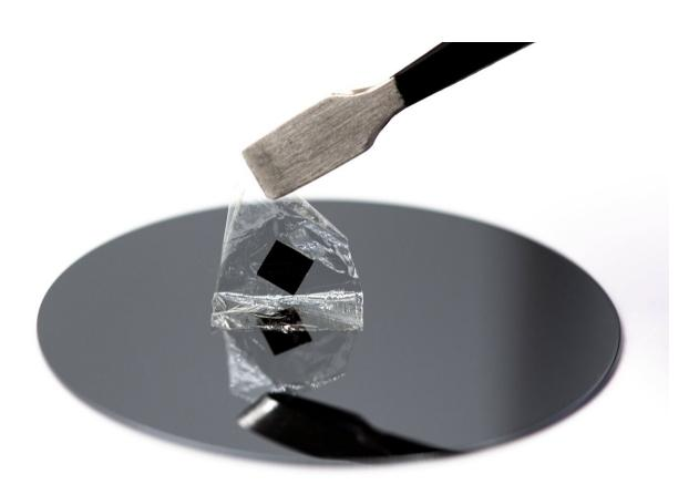
A single-crystalline perovskite thin film during the transfer process. Credit: Yusheng Lei
