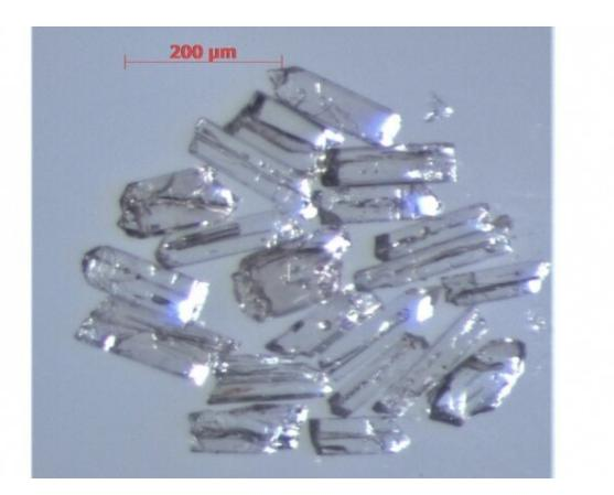
Microscopic crystals of the uranium-bearing mineral zircon were separated from the rock samples and analyzed by the U-Pb isotopic technique at the MIT Isotope Lab. These zircons yielded a precise age of  $221.82 \pm 0.10$  Ma for the upper Ischigualasto Formation. Credit: Courtesy of the researchers
