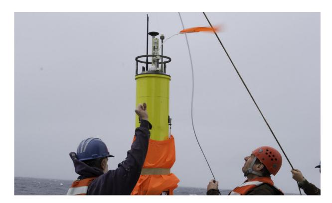
A research crew deployed a float from the R/V Knorr before releasing a fluorescent dye into the water. Scientists then tracked the drift of both dye and float through the Gulf Stream revealing significant mixing of waters across the swift current. Credit: Craig M. Lee, UW APL
