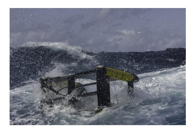
The "Triaxus" towing platform breaks through the choppy surface of the ocean during a storm. By towing such a platform with monitoring instruments through the water, changing its depth in a 'yo-yo' pattern as it traveled, scientists created high-resolution snapshots of how a dye released upstream evolved across the Gulf Stream front. Credit: Craig M. Lee, UW APL
