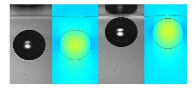
High-speed camera snapshots and simulations of bubbles bouncing from waterair interfaces can be used to detect trace amounts of contaminants. Credit: Ivan Vakarelski
