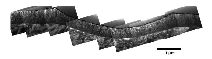
The material (thick gray line in the center of the image) derived from e-waste remained intact when indented, and increased the hardness of the steel below it. Credit: Adapted from *ACS Omega* 2020, DOI: 10.1021/acsomega.0c00485
