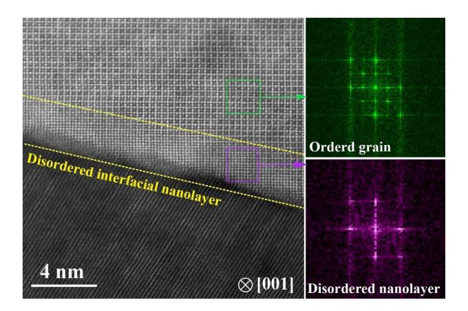
HAADF-STEM image reveals the ultrathin disordered layer at the grain boundaries with a thickness of about 5nm. Credit: *Science* DOI: 10.1126/science.abb6830
