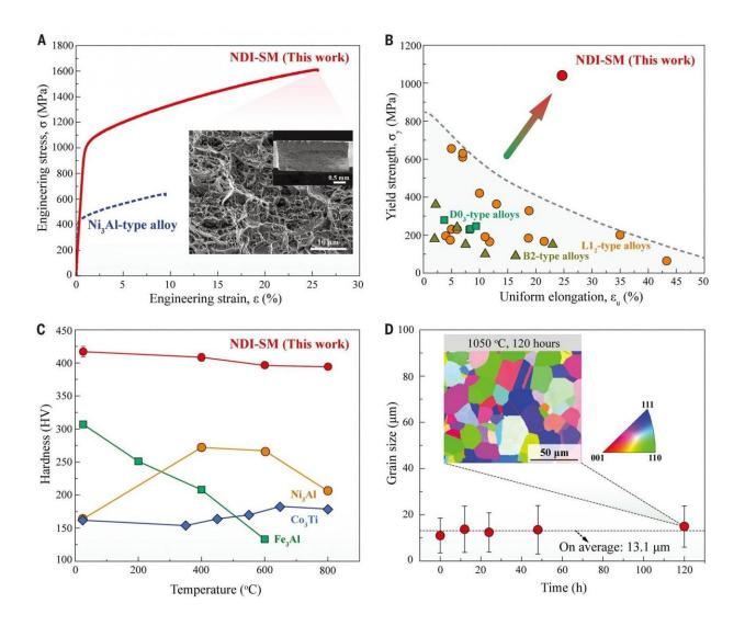
These pictures suggest that the alloy (NDI-SM) has achieved a superior strengthductility synergy at ambient temperature and extraordinary heat resistance at elevated temperatures. Credit: *Science* DOI: 10.1126/science.abb6830
