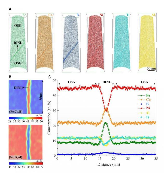
(A) Atom maps reconstructed using 3D-APT show the distribution of each element. Iron (Fe), cobalt (Co), and boron (B) are enriched (darker in colour) at the nanolayer, whereas nickel (Ni), aluminum (Al), and titanium (Ti) are depleted (lighter in colour) correspondingly. (B) and (C) also show the same results. Credit: *Science* DOI: 10.1126/science.abb6830
