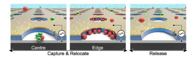
Model diagram of the nanogap electrodes allowing the dielectrophoretic tweezer technology. Credit: Korea Institue of Science and Technology(KIST)
