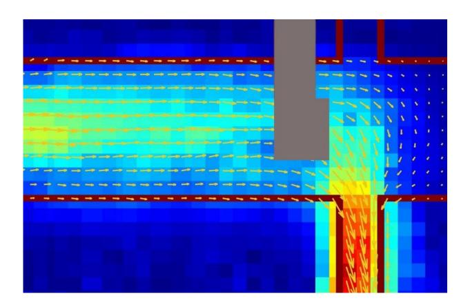
A picture of an electrical current in graphene (marked by the red outline) showing a fluid-like flow imaged using a diamond-based quantum sensor. The grey portion is where the metal electrical contacts prevented collection of data. Credit: Walsworth and Yacoby research groups, Harvard and University of Maryland
