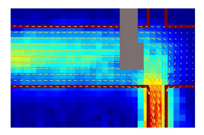
A picture of an electrical current in graphene (marked by the red outline) showing a fluid-like flow imaged using a diamond-based quantum sensor. The grey portion is where the metal electrical contacts prevented collection of data. Credit: Walsworth and Yacoby research groups, Harvard and University of Maryland
