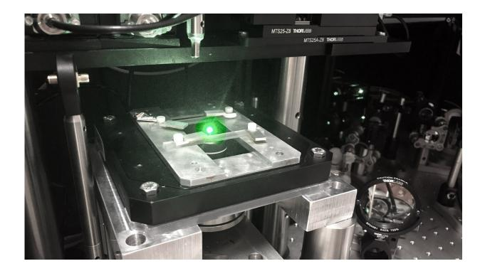
Microscope setup for capturing a 2D snapshot of a current in graphene via magnetic field imaging with nitrogen vacancies in diamond. The green light that excites NVs is visible in the image. (background color adjusted to highlight green light) Credit: Mason C. Marshall, Harvard and University of Maryland
