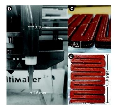
The paste is printed in shapes called material reactive architectures that determine how and where it burns. Credit: Vanderbilt University
