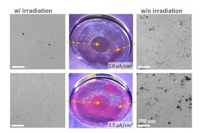
These optical and scanning electron microscope images show irradiated and unirradiated zones of a nickel-chromium alloy. The left side shows examples of foils with irradiation; instead of degrading the material as it almost always does, the radiation actually makes it stronger by reducing the rate of corrosion. Credit: Massachusetts Institute of Technology
